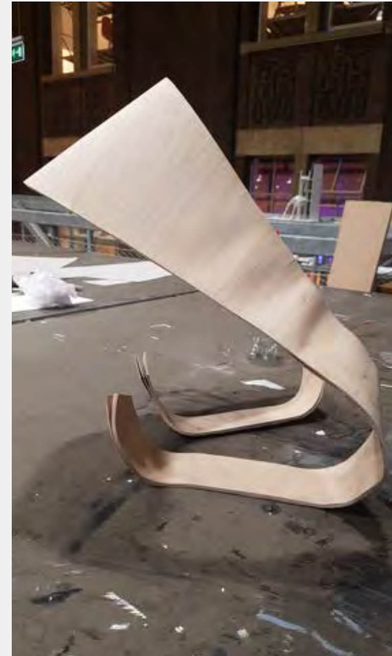
I printed a 'flattened' surface from the 3D model to use as a template. I used cork layers to help spread the load and bond the veneers evenly.
