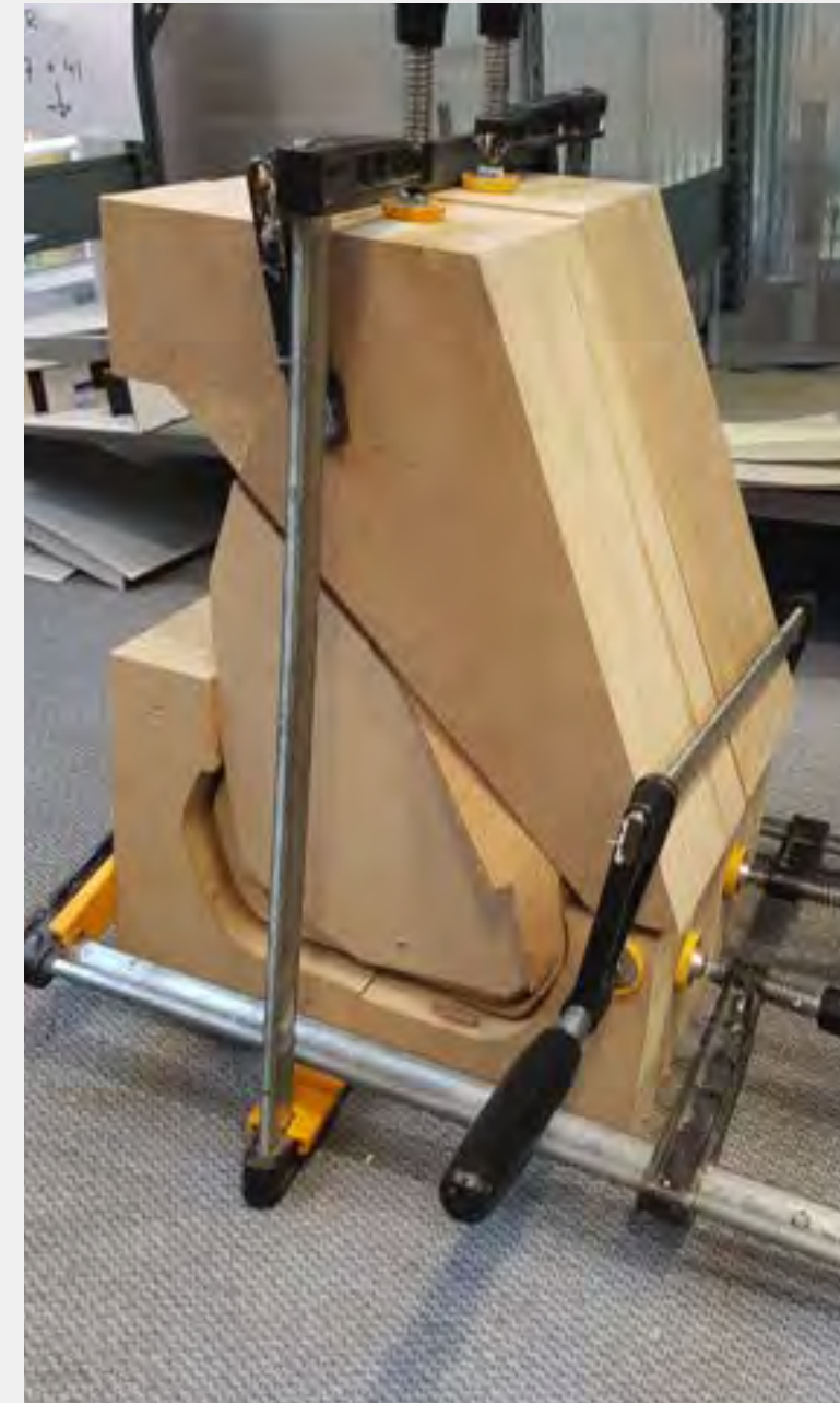
I printed a 'flattened' surface from the 3D model to use as a template. I used cork layers to help spread the load and bond the veneers evenly.
