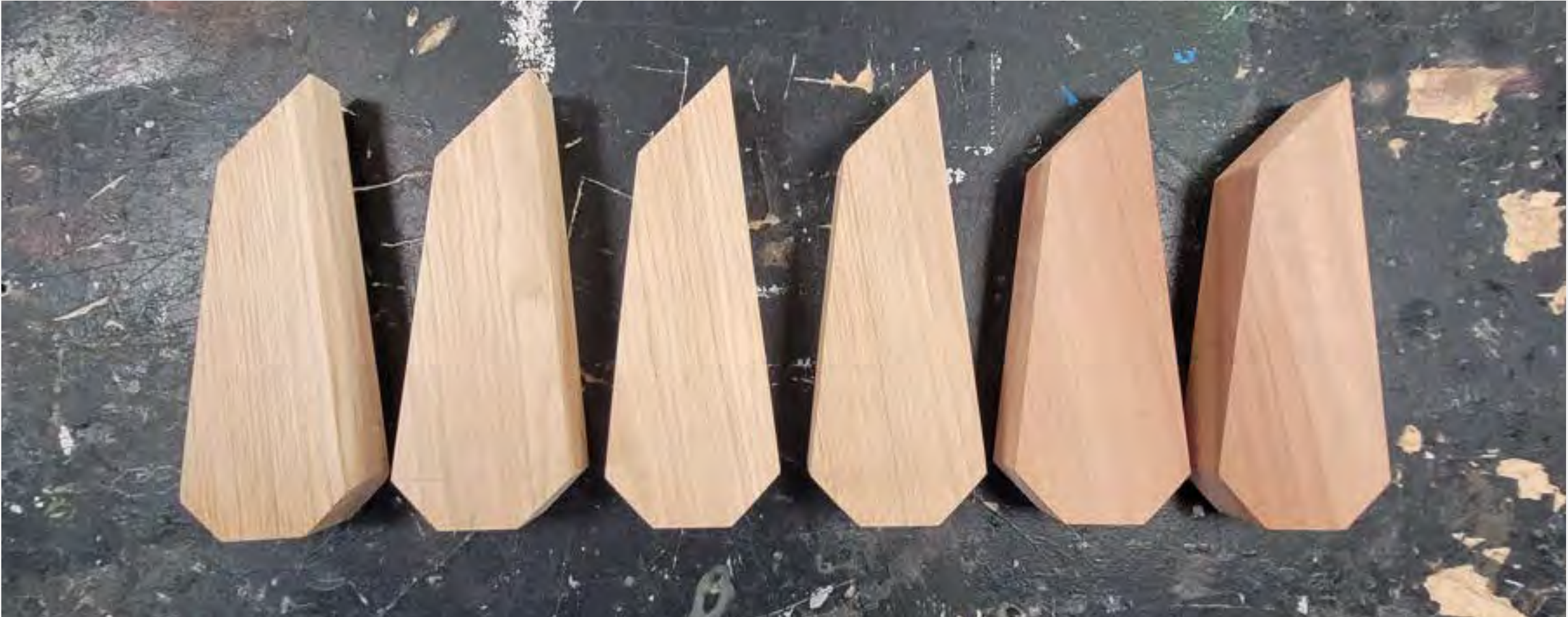
Prototyping the metal revealed inward angles couldn't be polished. I used the table saw and belt sander for the wood. To avoid a visible seam on the 'enhanced version' I used hand tools.
