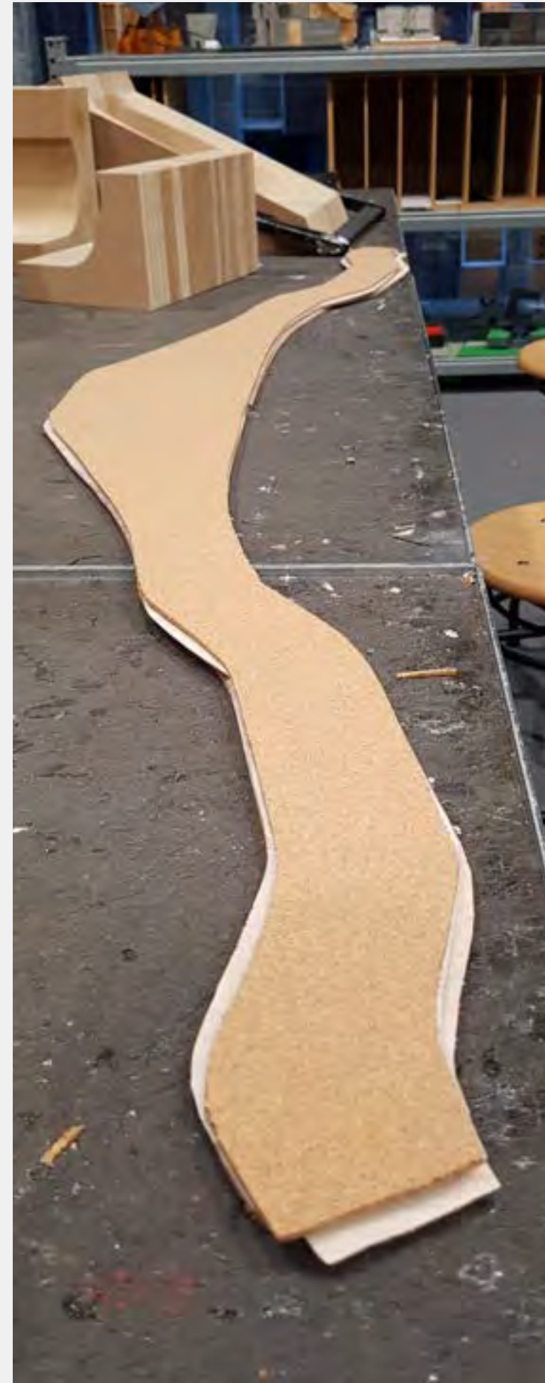
I printed a 'flattened' surface from the 3D model to use as a template. I used cork layers to help spread the load and bond the veneers evenly.
