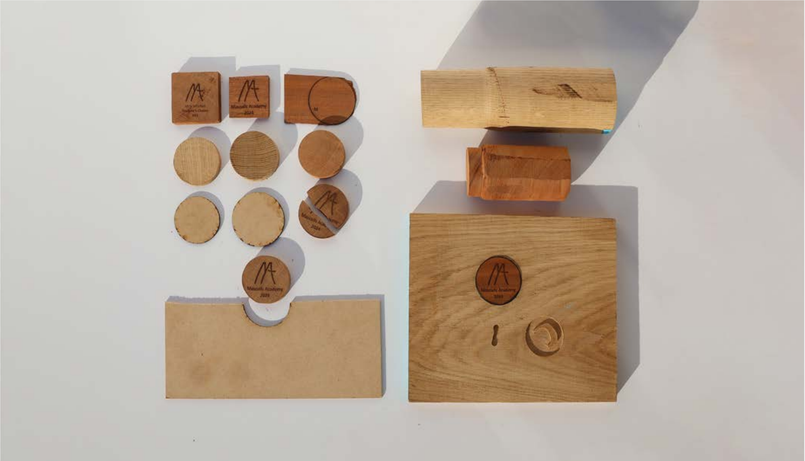
It was a challenge making disks that fit into holes perfectly. The best method was to turn the disks on the lathe and to use a router jig for the holes. Once they were flush, I engraved the text.
