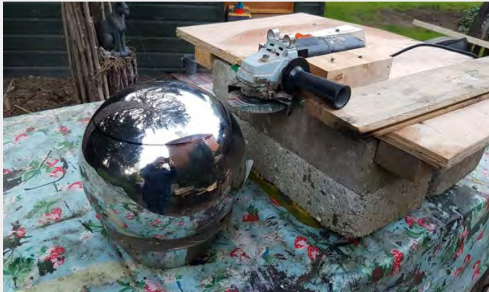
I made a jig for the angle grinder from a series of stiff objects to ensure a straight cut. I then rotated the sphere around slowly pushing it into the blade.
