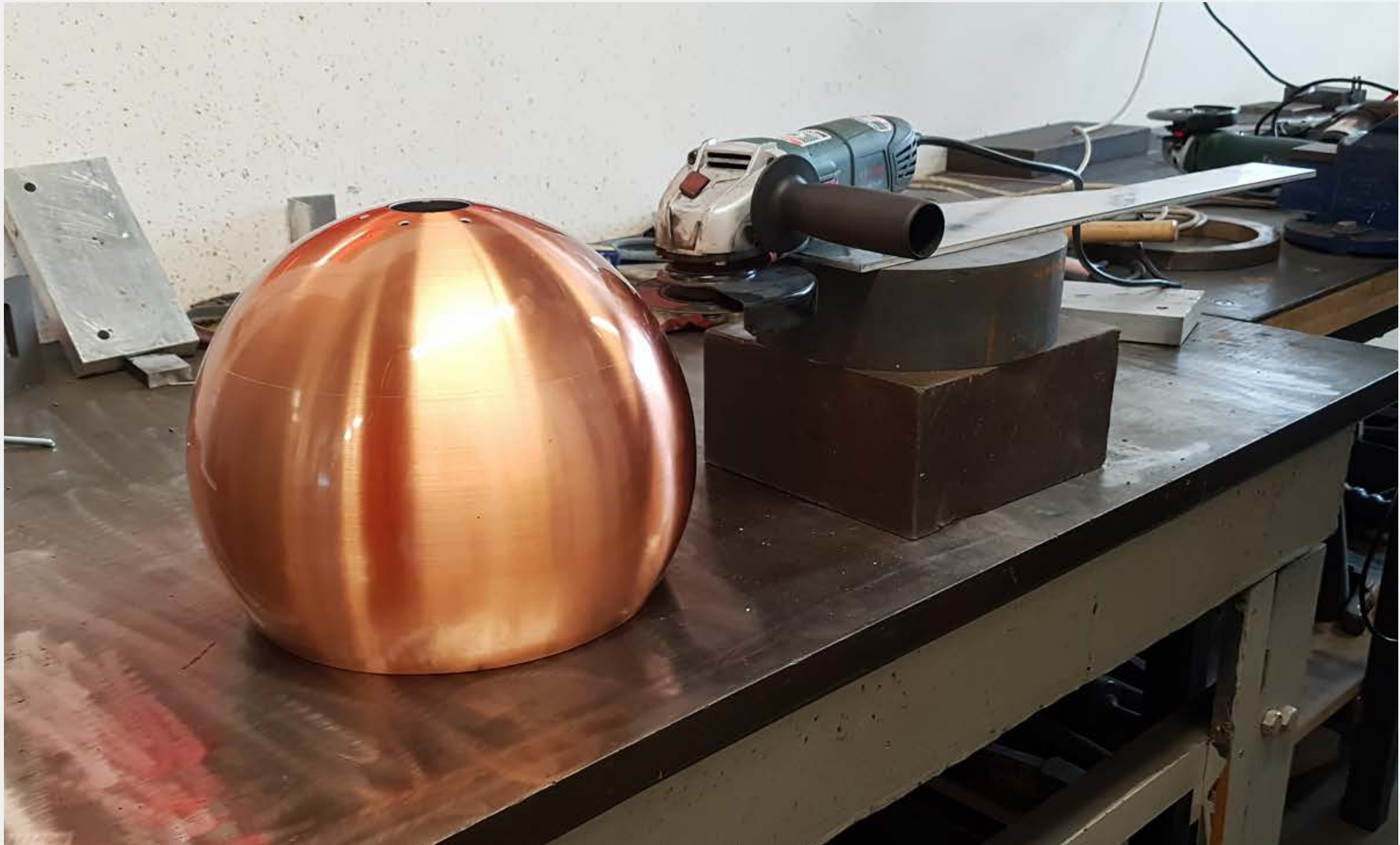
I made a jig for the angle grinder from a series of stiff objects to ensure a straight cut. I then rotated the sphere around slowly pushing it into the blade.
